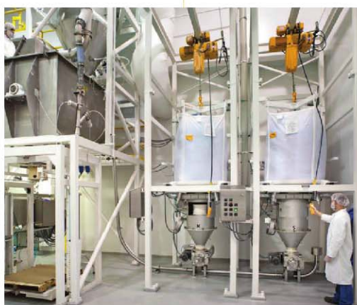
From each bulk bag, dry whole wheat flour and instant nonfat dry milk are pneumatically conveyed to a weighing hopper and then into a Munson double ribbon blender.
